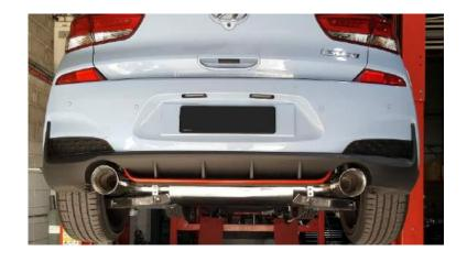
Note: When you first start your vehicle after the installation of your new XFORCE Performance Exhaust System, there may be some smoke and fumes coming from the system. This is a protective oil based coating used in the manufacturing of mandrel bent performance exhaust tubing. This is not a problem and will disappear within a very short period of time after the exhaust has reached normal operating temperatures.
