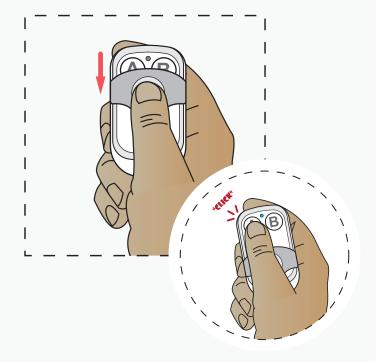
Slide the cover down to expose the buttons "A" & "B". Some remotes are callibrated to have open and close on either of those buttons, so test both to make sure you hear the varex motors operate on the vehicle before starting it.
